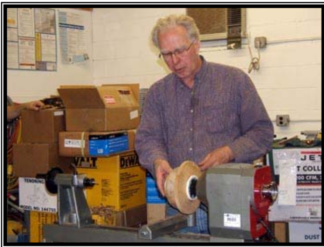
Finishing bottoms using jam chuck method
