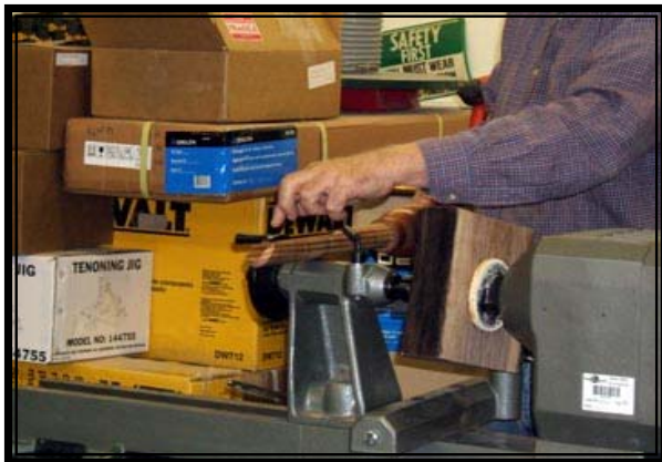
Ken demonstrating use of the Elsworth gouge – the flute is facing up.
