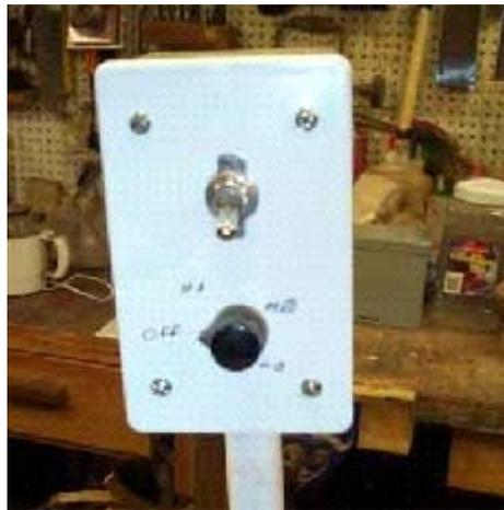
Motor and Controller Cooling: This is an important issue. Not so much the motor, because I turned for hours with this motor, touched it with my bare hand, and it would be cool to the touch, not a bit of warmth. However, the controller is another matter. There are two green voltage-reducing resistors, which get too hot to touch within 30 seconds of the power being turned on.
