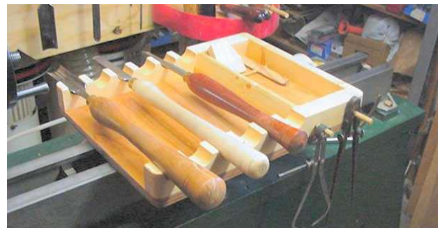
Handy Tool Tray slides onto lathe bed Mike Green
