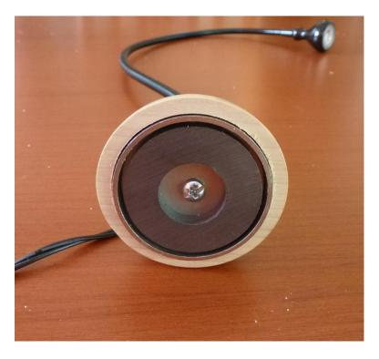
The lamp is ready for use on your lathe or other machine tool at this time, but the assembly is too top heavy to function on a non magnetic surface. I use the discarded weighted base now, by double sided taping the inside of the plastic cover to the weight, and then applying the pressure sensitive adhesive (PSA) felt to the bottom surface. When you want to use the lamp on a regular surface just place the weighted base and attach the magnetic base to the top of the plastic.
